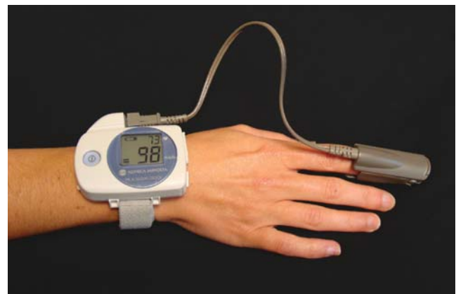
Figure 1 Pulsox-300i with finger probe (Finger Clip Probe SR-5C 0.3 m) used to assess oxygen saturation (Konica Minolta Sensing, Inc.).
